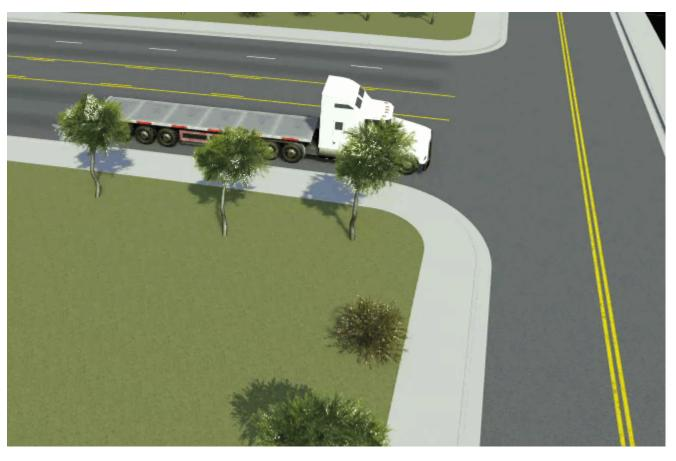
In the trailer vehicle attributes, set  $Connection \ Attributes > Type \ to \ fixed$ , this animation shows a sample truck with a trailer turning a corner with the trailer fixed to the truck.
